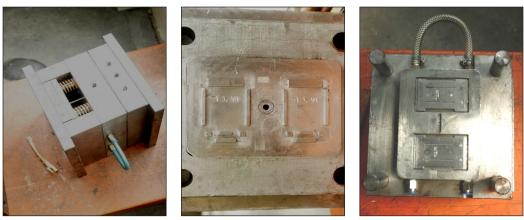
(a) (b) (c) *Figure 2.* (a) NTP mould set; (b) Female mould of NTP; and (c) Male mould of NTP
