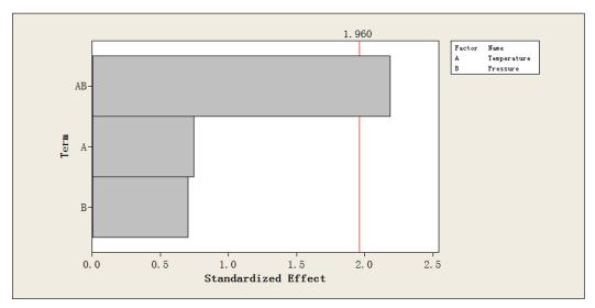
Figure 7. Pareto chart of NTP-filled PVOH/Starch (response is ln of weight SD, alpha= 0.05)
