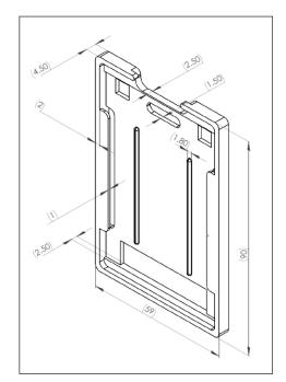
*Figure 1.* Drawing and measurement of NTP (unit in mm)
